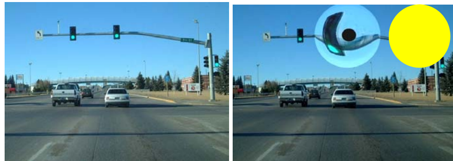
Figure 6. Left: A wide view of a scene by the video camera. Right: The same image processed for the position of the macula centered on the right edge of the traffic light. Black spot corresponds to foveola, where no cells will be stimulated. Pixels around the black spot are stretched radially in order to match retinal architecture (lighter circle). A white circle indicates a part of the display projected onto a photovoltaic battery located on retina aside the stimulating chip. The rest of the image represents a view through the transparent goggles for the remaining natural vision of the patient.
